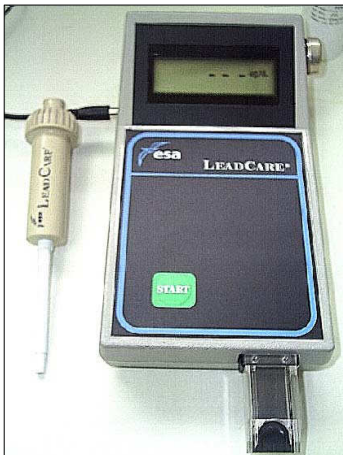
Annexure 4. The Lead Care blood lead analyzer
